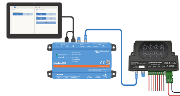
SmartSwitch DC4 connected at the end of the VE.Can network
